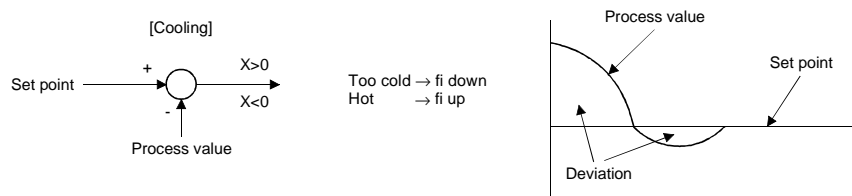
Relationships between deviation and manipulated variable (output frequency)
